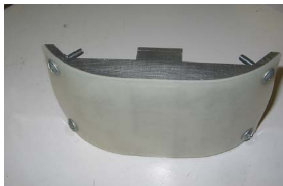
Test foot with clamping screws
