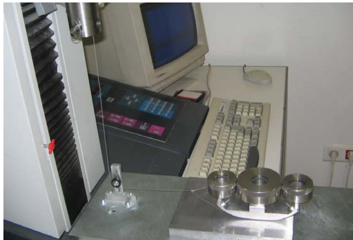
Determination of sliding distance force (note additional mass added to test foot)
